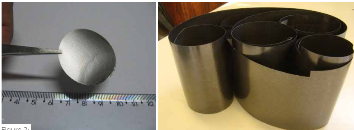
Figure 2: Highly flexible conductive thin-films, manufactured from graphene nanotapes. Cooperation: Nacional de Grafite
