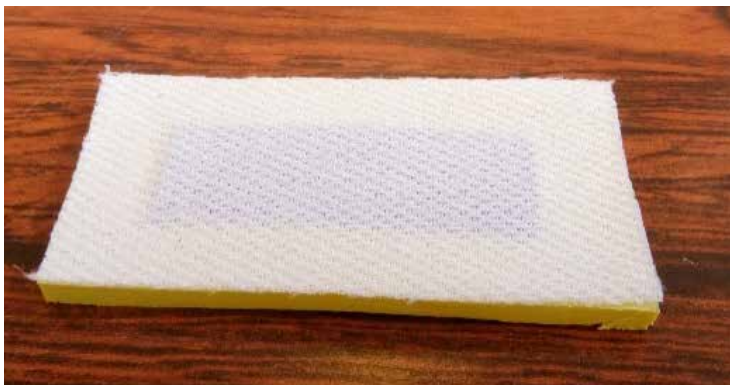
Figure 4: Sandwich-like structure of the insole material, material (function), from top to bottom: fabric (protection)/thermo-fixation film (fixation)/conductive film in nanographite (heating) / thermo-fixation film (fixation) / EVA film (dampening). Cooperation: Dublauto
